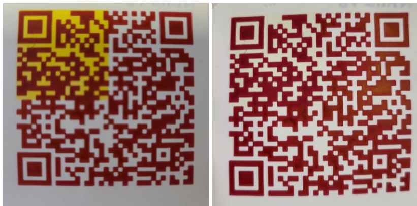
Figure 3: A principle of a smart tag for DPPs: (a) a standard QR code is combined with a sensor area (yellow area in the top left corner) that (b) changes its colour (from yellow to transparent) when exposed to a threshold value of a condition it is sensitive to (in this case > +37 °C).
